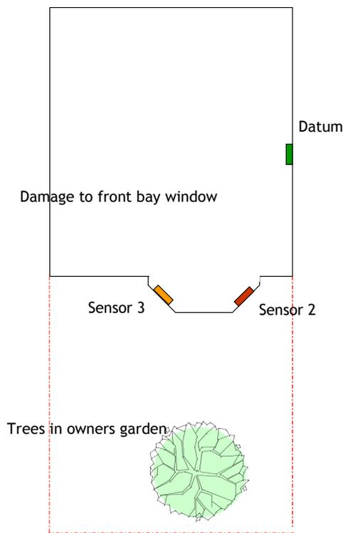
The datum shows movement of 0.07 degrees. In contrast the sensors fitted to the bay window have recorded movement of 0.13 (Sensor 2) and 0.15 (Sensor 3) degrees.
